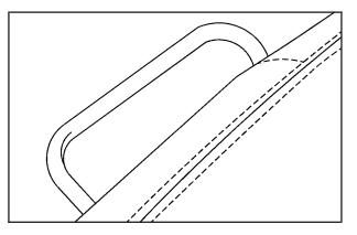
Your vehicle may have manual seats. To adjust the seat, lift the bar under the front of the seat to unlock it. Slide the seat to where you want it and release the bar. Try to move the seat back and forth with your body to be sure the seat is locked in place.
